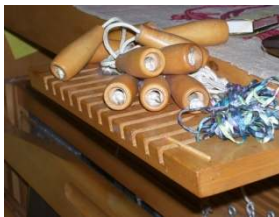
Draw tie-up for Clement loom
