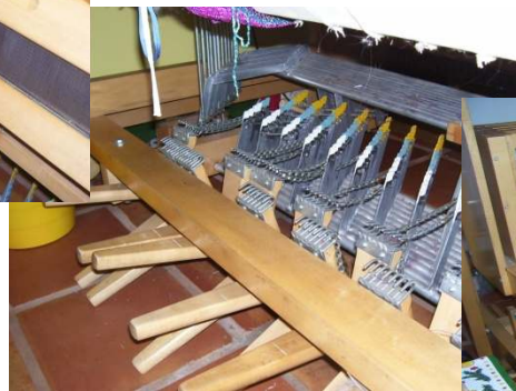
Clement unique chain tie-up and ergonomic treadles
